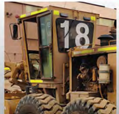
Equipment ID Decals
