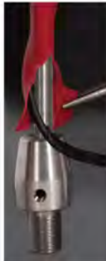
Red Sheathing cut away to show rod
