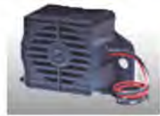
HM-B/U-alarm 107db Backup Alarm, 107db This compact, high sound level alarm is specifically designed for 107 decibels. This solid state alarm is polarity protected. The 270 alarm has an approximate current draw of 0.5 Amps. Self-resonating circuitry automatically adjusts to environmental conditions to ensure a constant 107 decibel output. Weight: 12 oz. (340 g)
